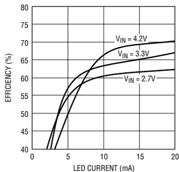
Figure 8. Li-Ion white LED driver efficiency
