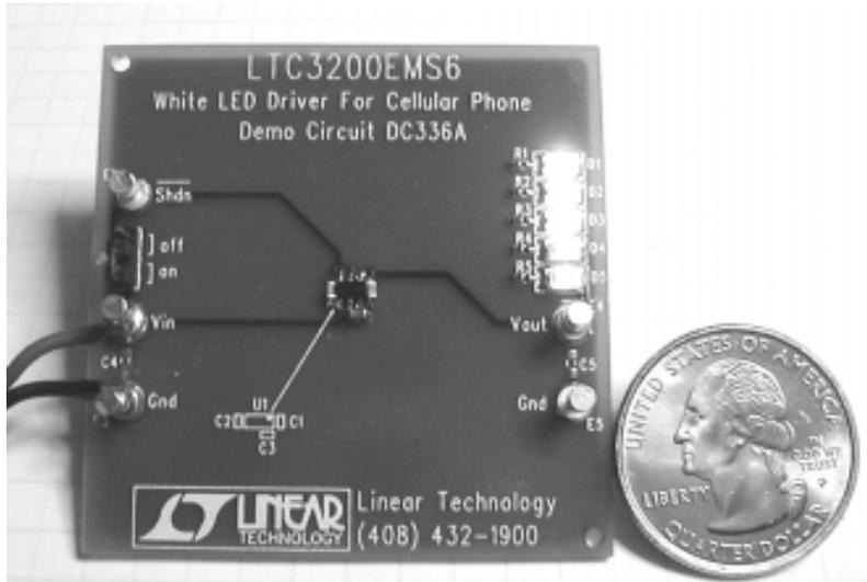
Figure 1. LTC3200 evaluation circuit
