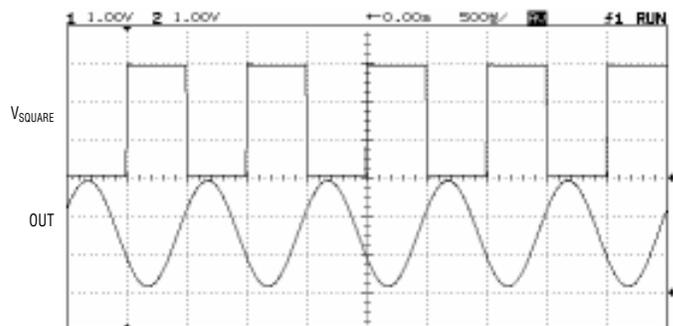
**Figure 7. Scope capture for a 100kHz tone ( $R_{SET} = 158\text{k}$ )**
