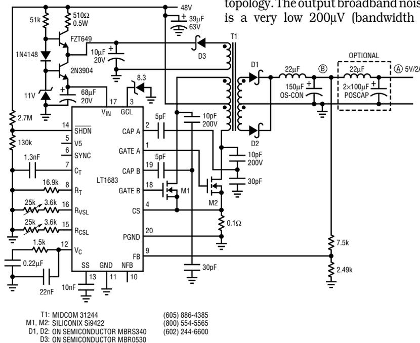
Figure 1. Ultralow noise 48V to 5V DC/DC converter
