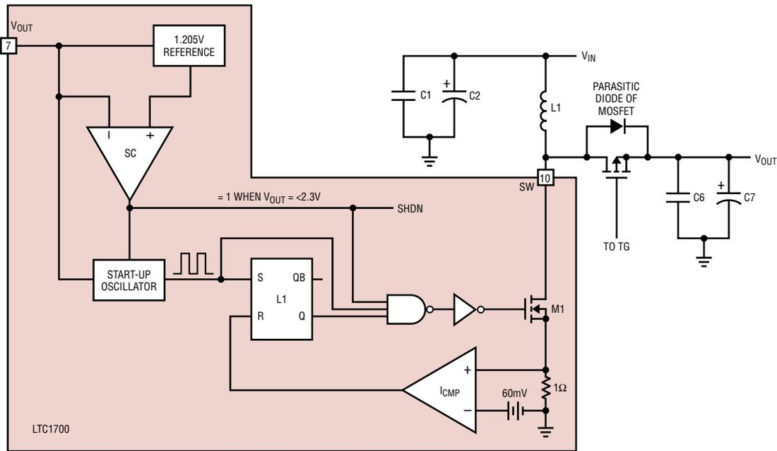
Figure 4. Start-up components of the LTC1700
