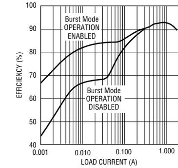
Figure 10. Efficiency of Figure 9's circuit
