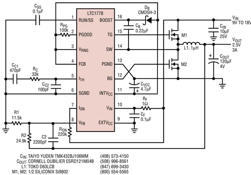
Figure 6. 2.5V/3A converter switches at 1.4MHz
