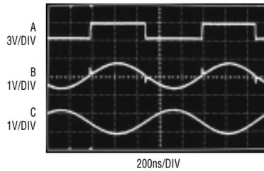
**Figure 6. Oscillator waveforms with  $V_S = 3\text{V}$ : Trace A = comparator output; Trace B = crystal feedback to pin 2 of the LT1713; Trace C = buffered, inverted and bandpass filtered output of LT1806**
