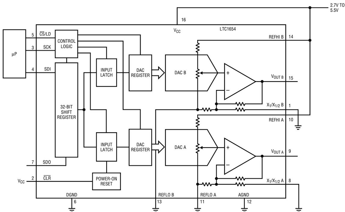
Figure 1. LTC1654 block diagram
