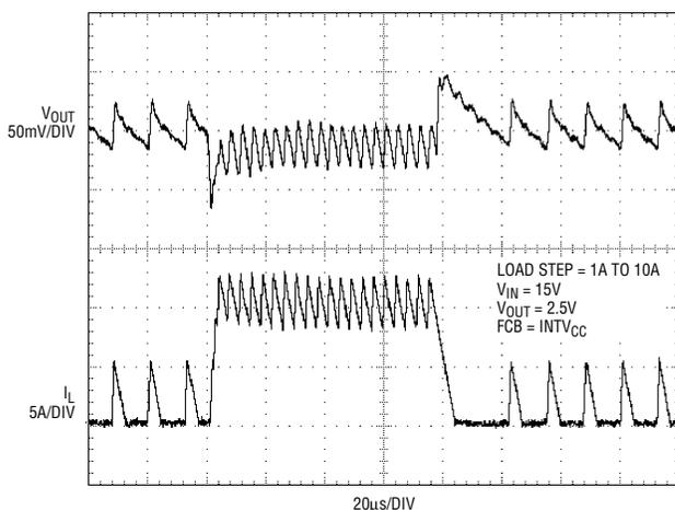
Figure 5. Transient response of Figure 3's circuit
