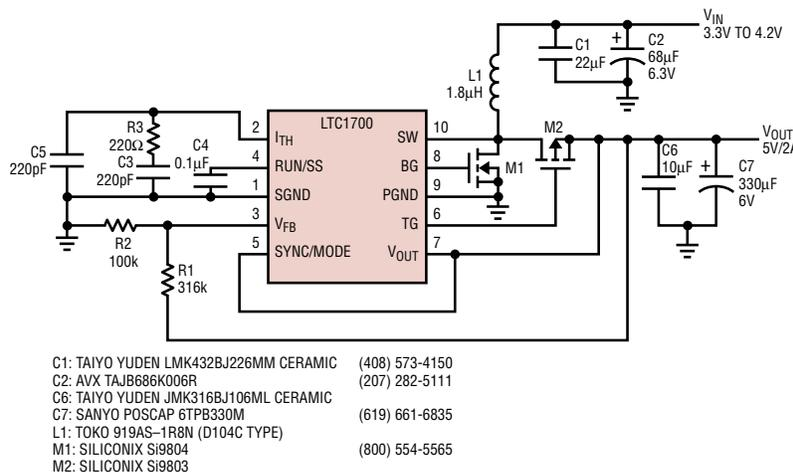
Figure 1. 3.3 to 4.2V input, 5V/2A output converter
