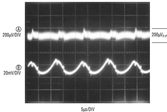
Figure 3. 5V output noise (bandwidth = 100MHz)
