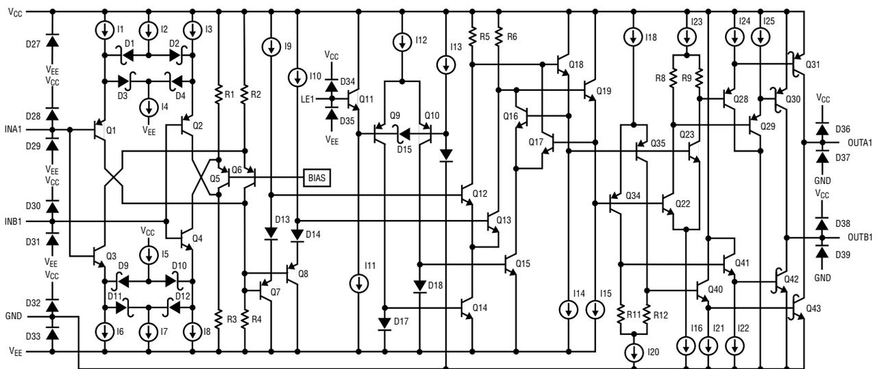
Figure 1. LT1711-LT1714 simplified schematic
