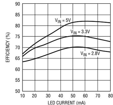
**Figure 10. High power white LED driver efficiency**
