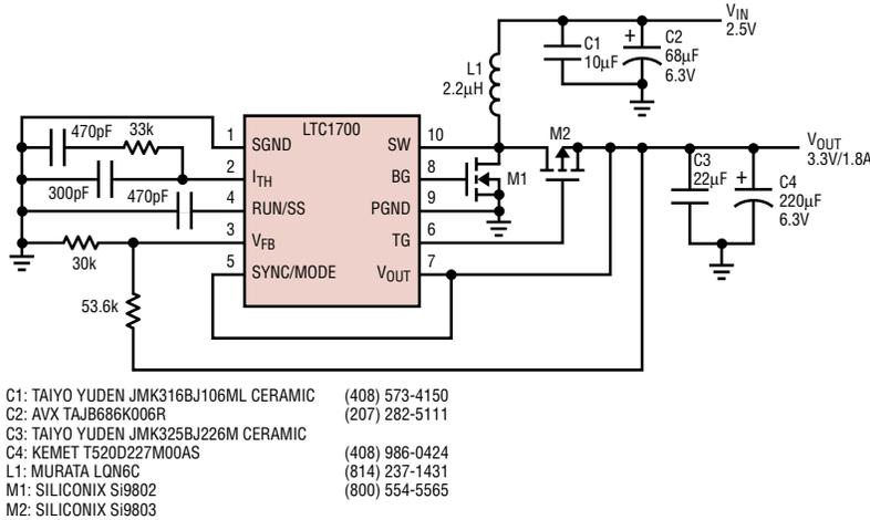
Figure 9. 2.5V input, 3.3V/1.8A output regulator
