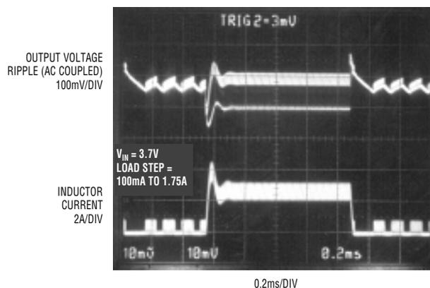
Figure 3. Load-step response of Figure 1's circuit
