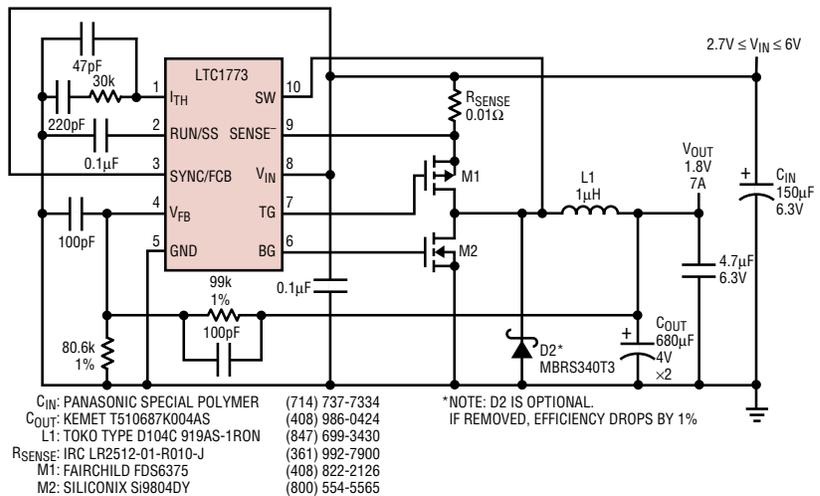
Figure 4. 3.3V to 1.8V/7A regulator
