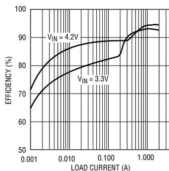
Figure 2. Efficiency of Figure 1's circuit
