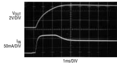
Figure 4. USB to 5V SEPIC during start-up
