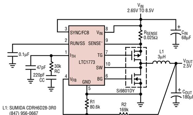
Figure 1. 5V to 2.5V/3A step-down converter
