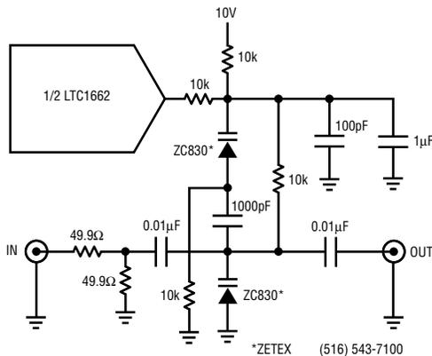
**Figure 2c. Low distortion phase control**
