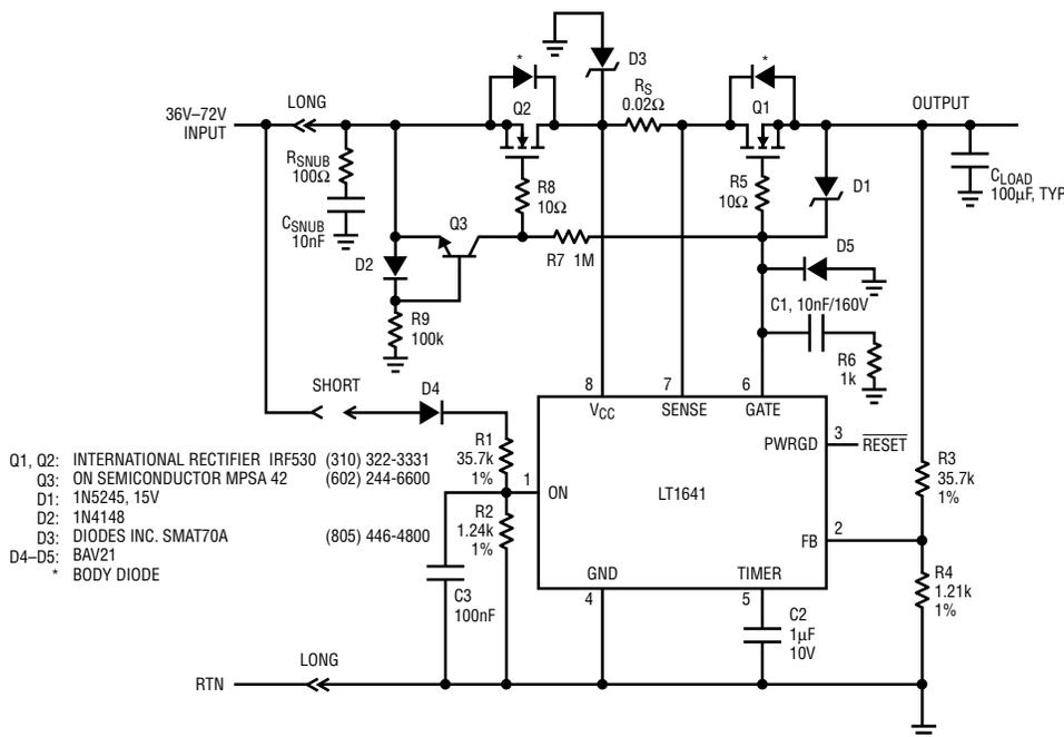
Figure 1. Reverse-battery protected LT1641 48V Hot Swap circuit
