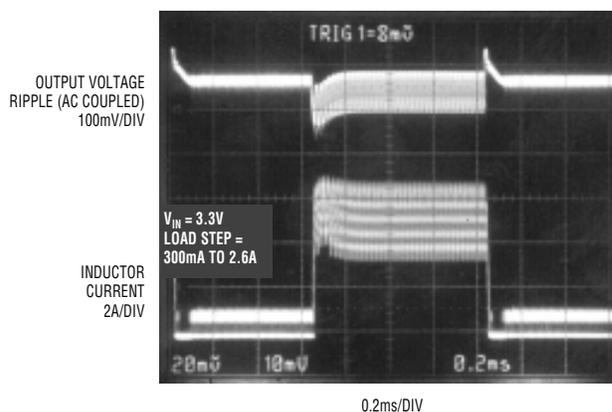
**Figure 7. Load-step response of Figure 5's circuit**
