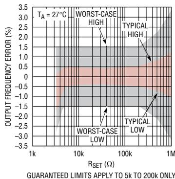
**Figure 2. Accuracy of the output frequency equation**
