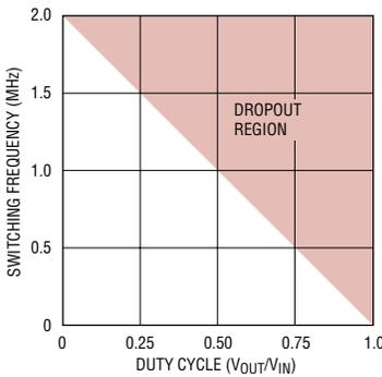
Figure 2. Maximum switching frequency vs duty cycle
