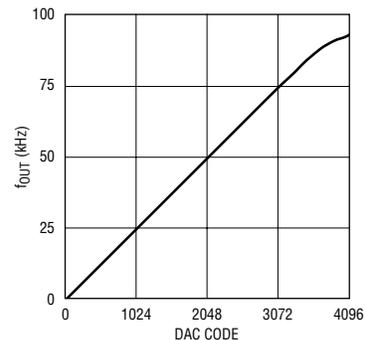
Figure 9. Input code vs output frequency for Figure 8's circuit
