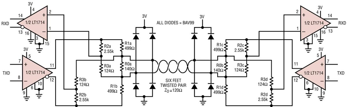
Figure 2. 75MBaud full-duplex interface on two wires
