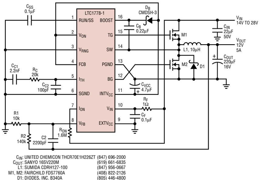
Figure 7. 12V/5A converter switches at 300kHz
