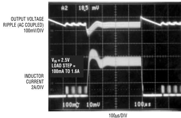
Figure 11. Load-step response of Figure 9's circuit
