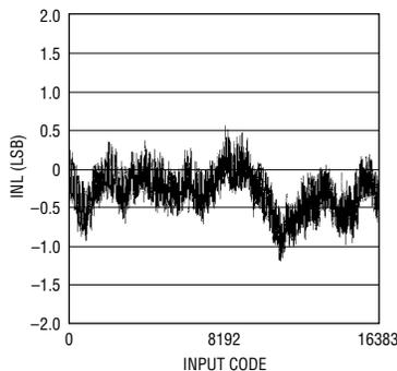
Figure 2. LTC1654 typical integral nonlinearity (INL)
