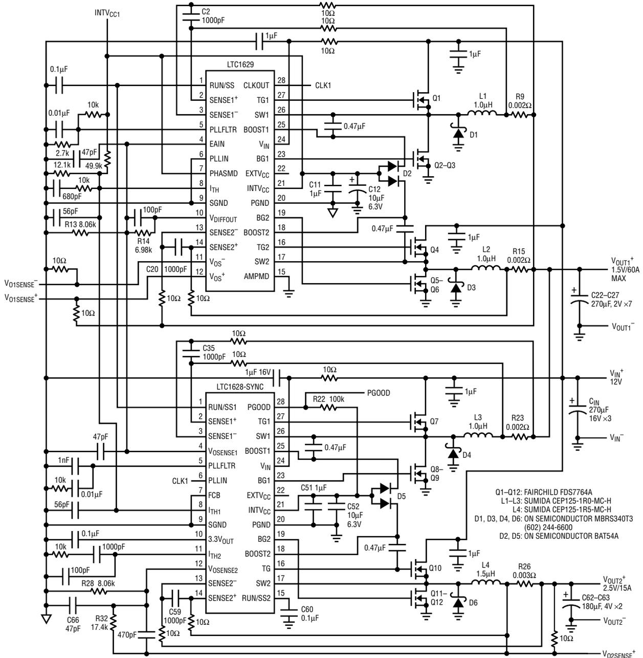
Figure 1. LTC1628-Sync/LTC1629 2-output PolyPhase supply
