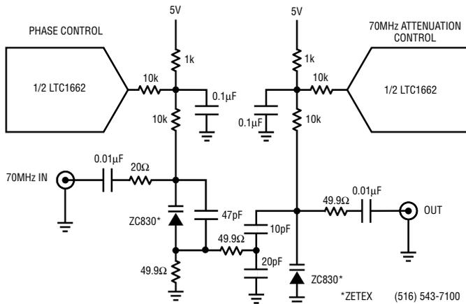
**Figure 2a. 70MHz attenuation control**
