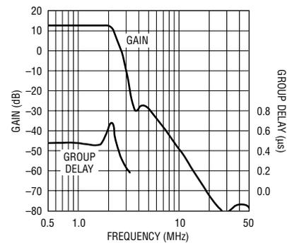
Figure 1. LTC1566-1 gain and group delay vs frequency
