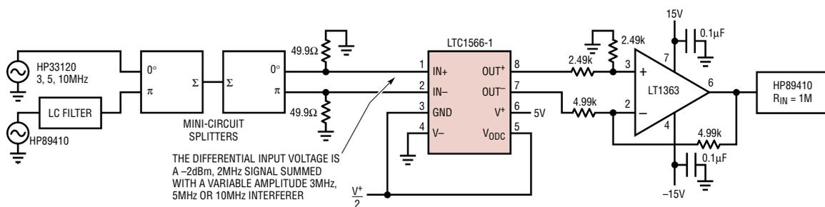
**Figure 8. Test circuit for out-of-band rejection**
