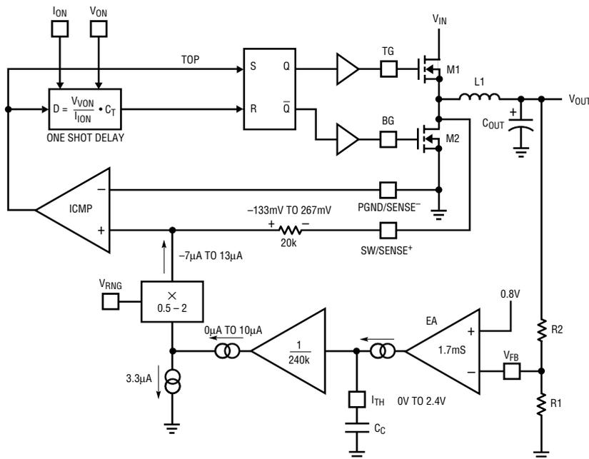
Figure 1. LTC1778 main control loop
