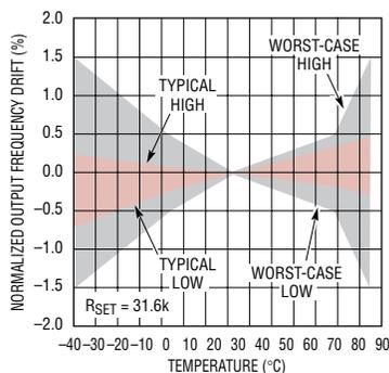
**Figure 3. Output frequency temperature drift**
