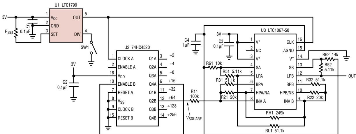
**Figure 6. 80Hz to 8kHz sine wave generator**
