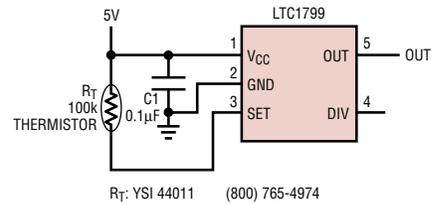
**Figure 4. Temperature-to-frequency converter**
