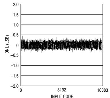
Figure 3. LTC1654 typical differential nonlinearity (DNL)
