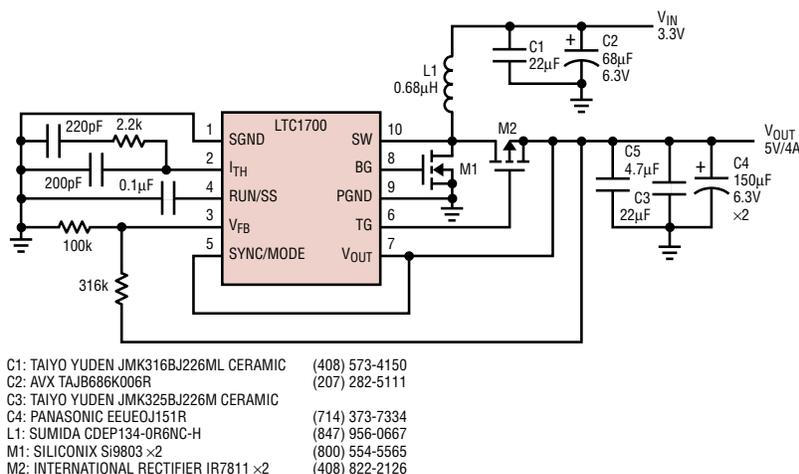
**Figure 8. 3.3V input, 5V/4A output regulator**
