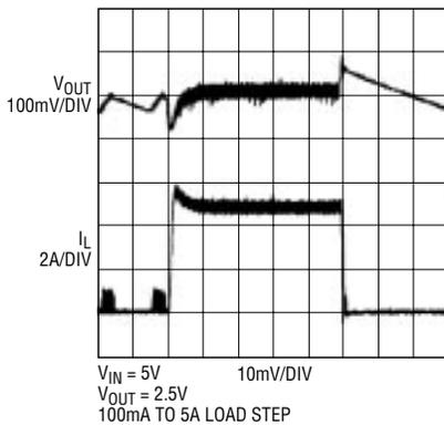
**Figure 3a. Load-step response, Burst Mode operation**
