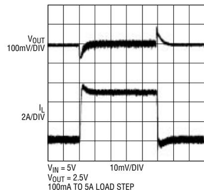
**Figure 3b. Load-step response, continuous mode operation**
