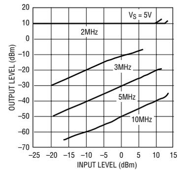
**Figure 9. Out-of-band rejection,  $V_S = 5V$**
