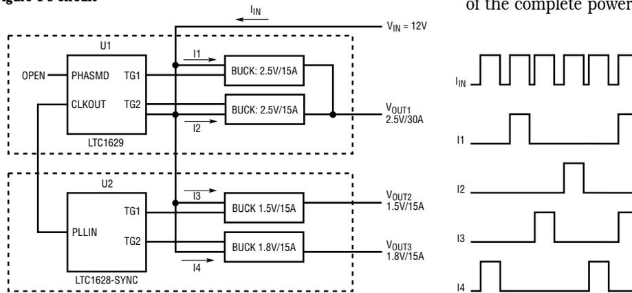
**Figure 3. Block diagram of LTC1628-Sync/LTC1629 3-input, 4-phase application**
